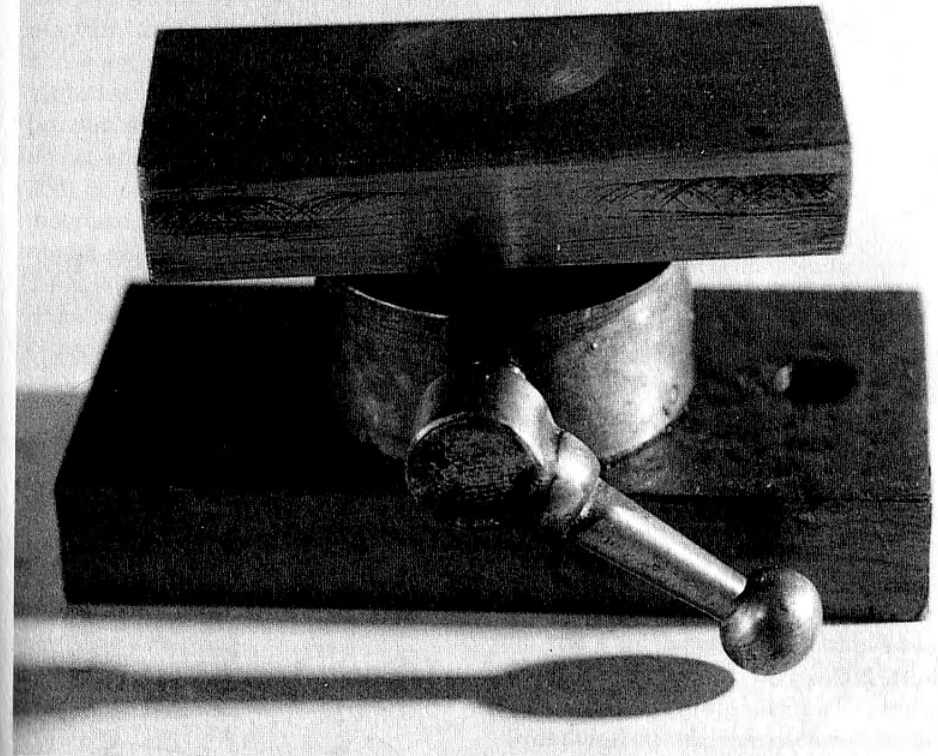
The hand turning rest seen from the rear. It consists of only two basic parts, both of which are fabricated.
